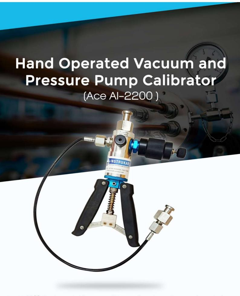
Ace AI-2200 Hand operated Pressure and Vacuum Pump is easy to use and operated manually with a pressure generation of 30 Bar and vacuum upto -0.9 Bar. This pneumatic hand pump calibrator is economical and accommodates most digital gauges as master for calibration and comparison purposes
